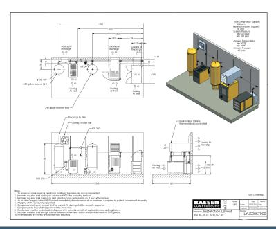
If new equipment is warranted, we can provide detailed drawings for installation planning to ensure proper pipe sizing and storage as well as adequate ventilation.
